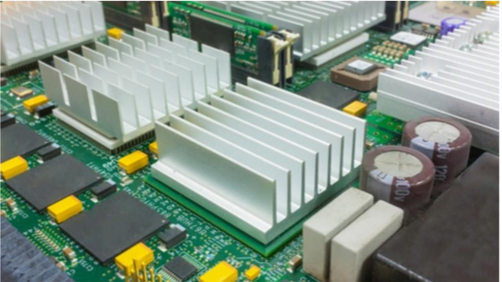
Aluminium Heat Sink are produced from a solid block of metal. These heat sinks offer high design flexibility and you can achieve high fin-density. This creates more surface area and opportunity for heat dissipation. They offer medium to high performance, but their drawbacks are generally high weight and directional sensitivity.
