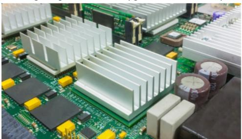
Aluminium Heat Sink are produced from a solid block of metal. These heat sinks offer high design flexibility and you can achieve high fin-density. This creates more surface area and opportunity for heat dissipation. They offer medium to high performance, but their drawbacks are generally high weight and directional sensitivity.
